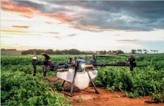
← New Holland, a CNH Industrial brand, develops agricultural drones, including the FieldXplorer, which allows farmers to take aerial images of their fields to identify and treat areas with weed or disease problems.
