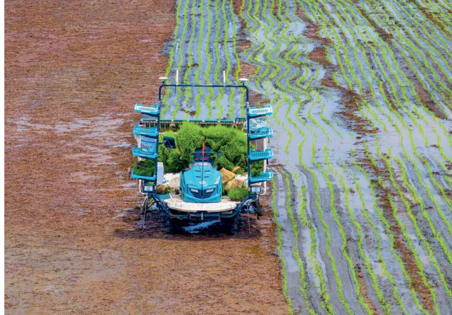
↑ An autonomous rice transplanting machine transplants seedlings in a rice paddy in Zhaohe, eastern China, in June 2024.
