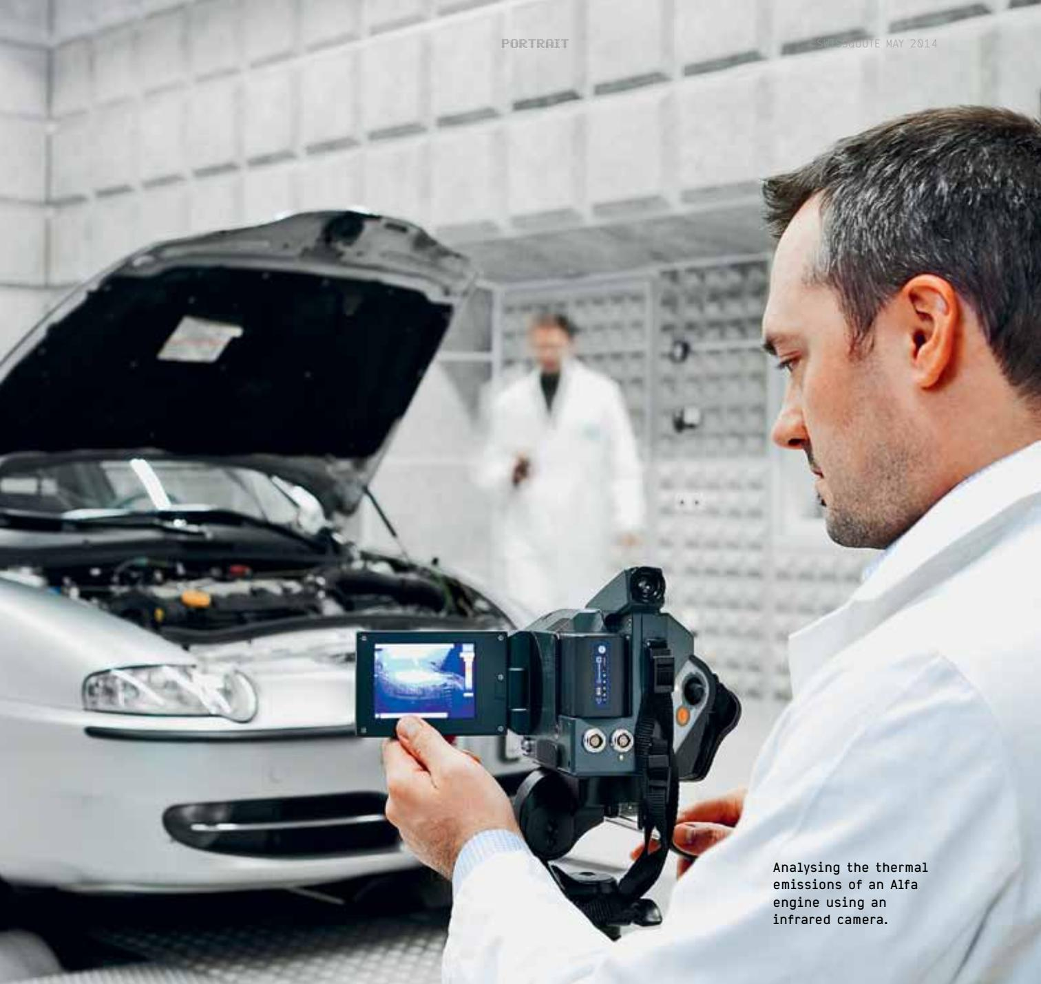
Analysing the thermal emissions of an Alfa engine using an infrared camera.
