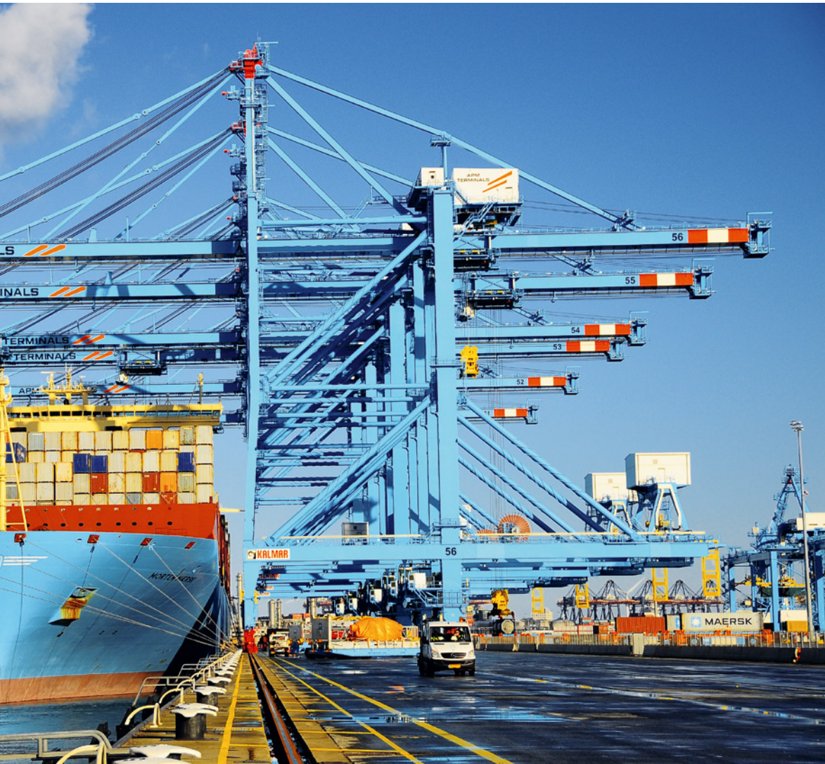
The terminal of APM Terminals in Maasvlakte 2. The eight automated unloading cranes are operated remotely.
