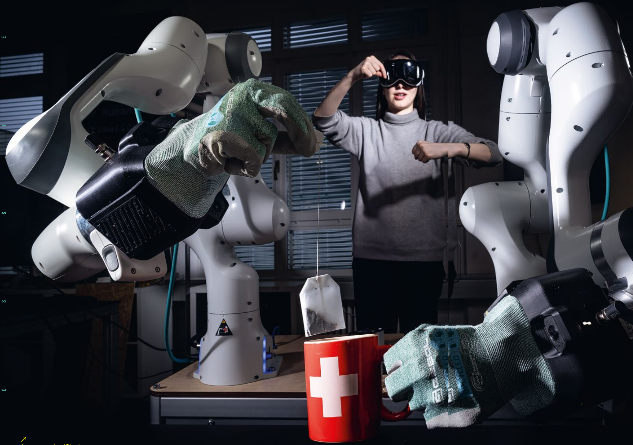
➤ An operator wearing a VR headset guides the robot's movements during a learning phase. Once trained, the robotic hand can reproduce the gestures autonomously.
