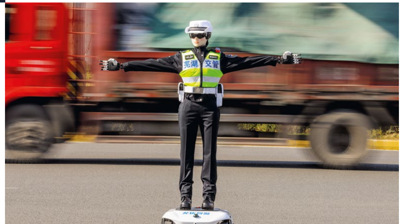
Photographed here in January 2026, the ‘Intelligent Police Unit R001’ robot is currently being tested in the city of Wuhu, China, to improve traffic flow. Equipped with high-definition cameras, this robot is capable of autonomously identifying traffic violations by non-motorised vehicles and pedestrians and issuing warnings to offenders. ↓
